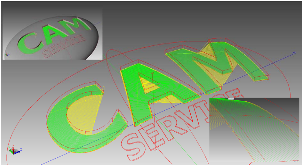
Pic 5: 3D hatching of curved faces using outer loops (sky writing) and random orientation for multiple planes by CAGILA® 3D
